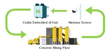
Accurately measured moisture in aggregates allows the concrete producer to optimize strength, durability, and shrinkage of concrete products without overdosing cement and increasing the cost of production and CO2 emissions.
